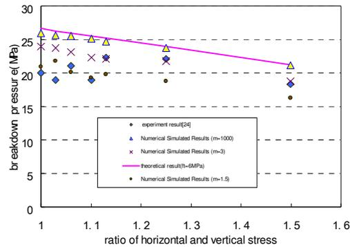
Figure 10: breakdown pressure with different pressure ratio( $\sigma_v / \sigma_h = 1.0-1.5$ )
