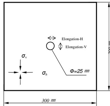
Figure 4: Sample geometry for simulating hydraulic fracturing [16]
