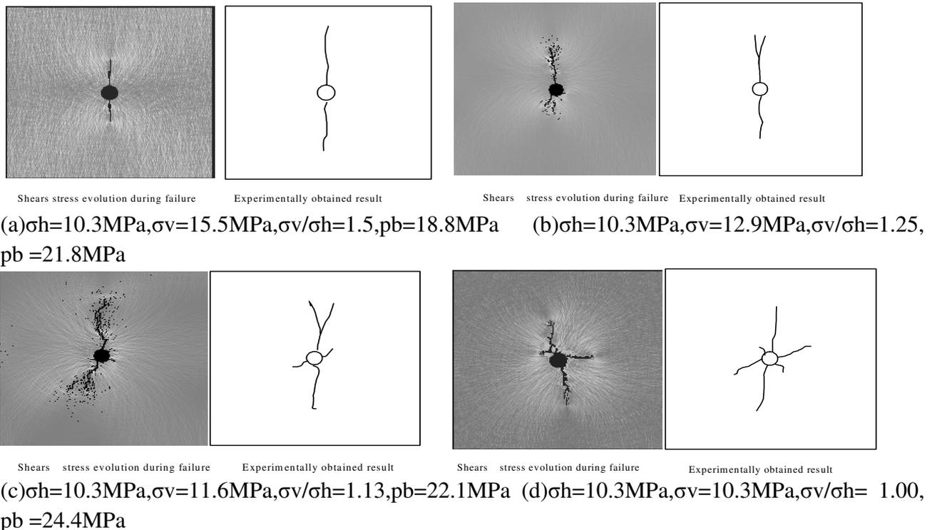
Figure 9: Experiment [17] and Numerical Simulated Results with different pressure ratio.
