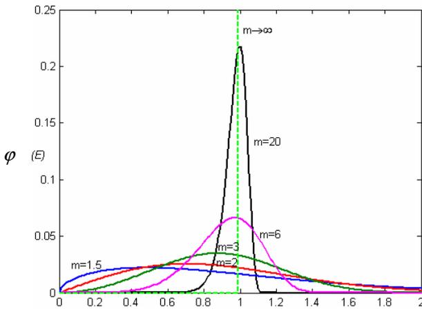
Figure 1: Weibull's distribution for rock specimens with different homogeneous
