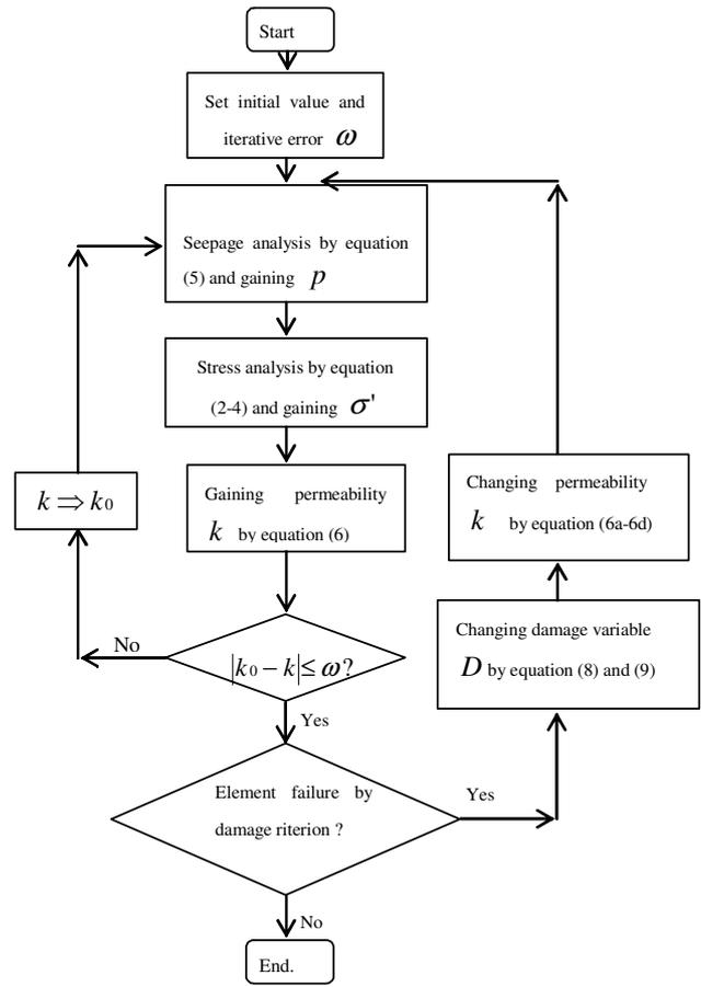
Figure 2: The flow chart of F-RFPA2D Program under uniaxial compressive stress and tensile stress
