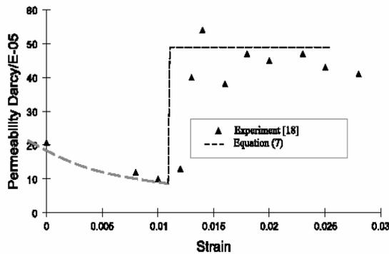
Figure 3: comparison of the permeability-strain experimental obtained by Yang [18] and equation (6)
