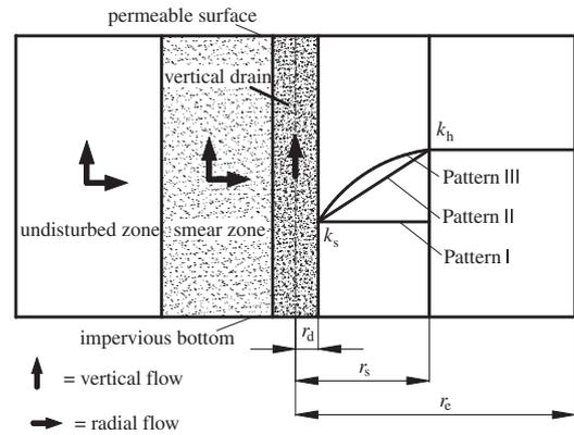
Fig. 2. A typical unit cell selected for modeling the consolidation of a vertical drain and three decay patterns of the horizontal permeability coefficient of the smeared soil toward the drain.
