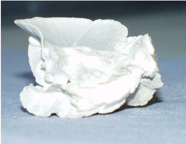
Fig. 13. Horizontal fracture created by high injection rate test [9].
