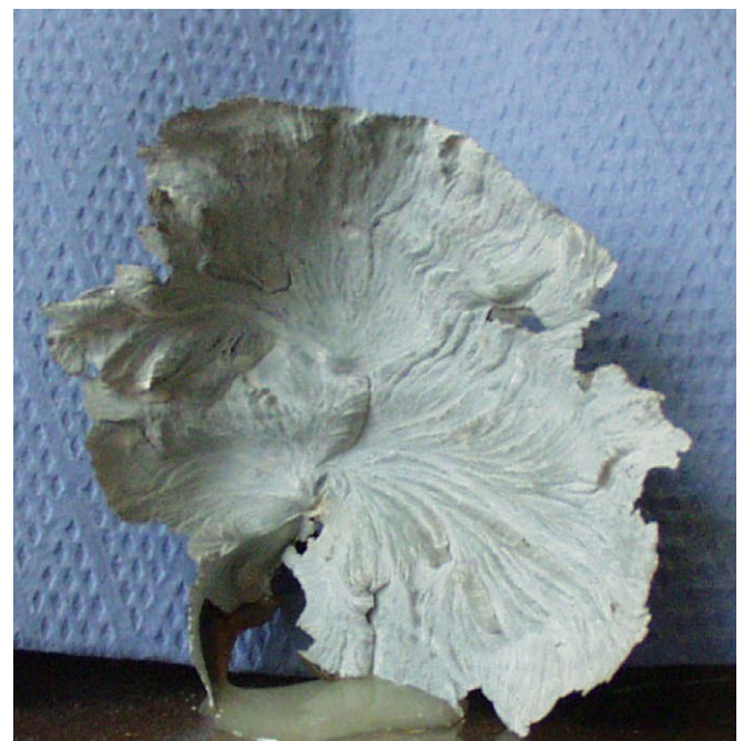
Fig. 12. Vertical fracture created by low injection rate test [9].
