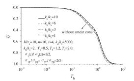
Fig. 5. Influence of reducing the horizontal permeability within the smear zone on the average degree of consolidation (Pattern III).
