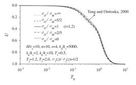
Fig. 4. Influence of the top to bottom stress ratio on the average degree of consolidation (Pattern III).
