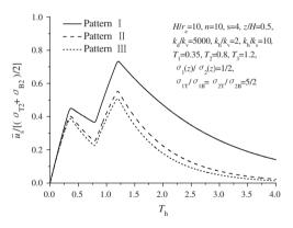
Fig. 3. Dissipations of the excess pore water pressure predicted with various decay patterns of the horizontal permeability of the surrounding soil.
