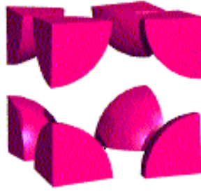
Fig. 2: 3D equal spheres size in a Simple Cubic arrangement.
