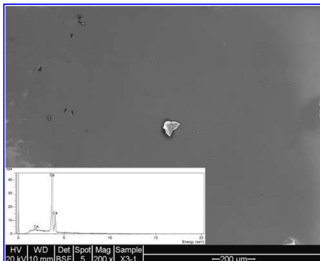
FIG. 7. SEM image (EDS spectra inset) of Iceland spar calcite exposed to PO_4^{3-} (as potassium phosphate).
