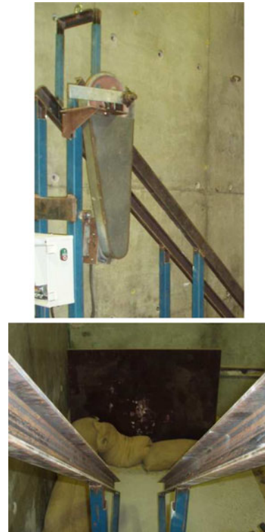
Fig. 2 Photographs of the testing apparatus. Top view of the top part of the ramp: spinning device with cover and release mechanism. Bottom view of the steel channels making the ramp
