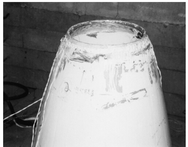
Fig. 9. Failure under axial compression.
