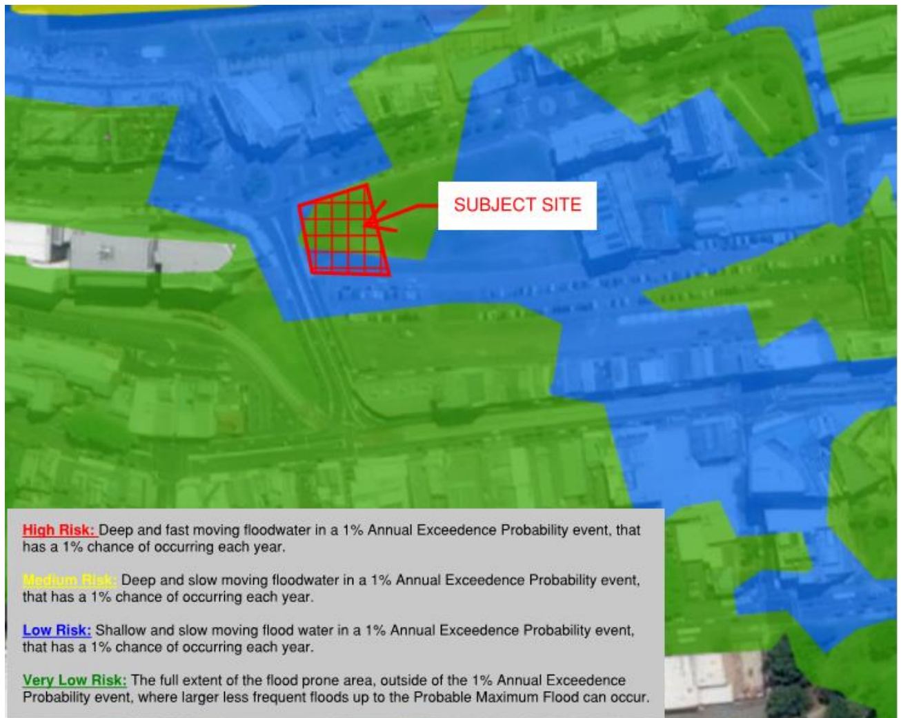
Figure 4 – Local catchment flood behaviour (The City of Newcastle Online Interactive Flood Maps)
