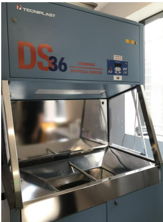
Waste disposal station in PC2 zone
