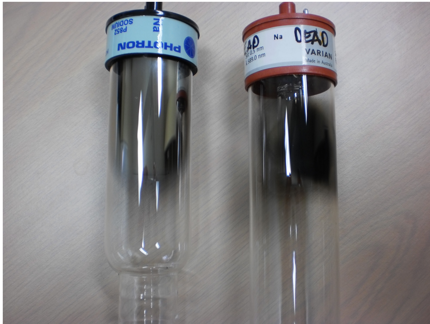
Figure 1: A new AAS lamp (left) and a burnt out old AAS lamp (right)
