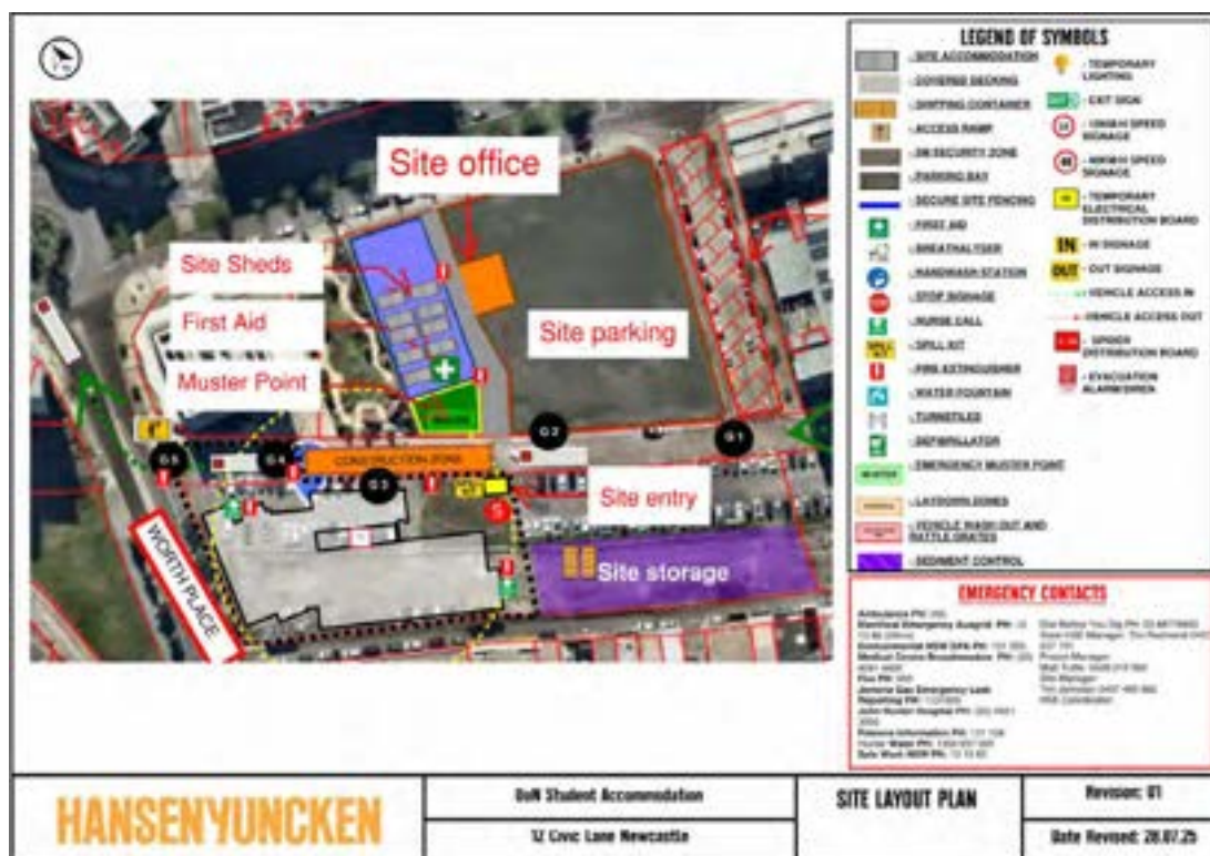
Figure 3 – Site and Traffic Management Plan
