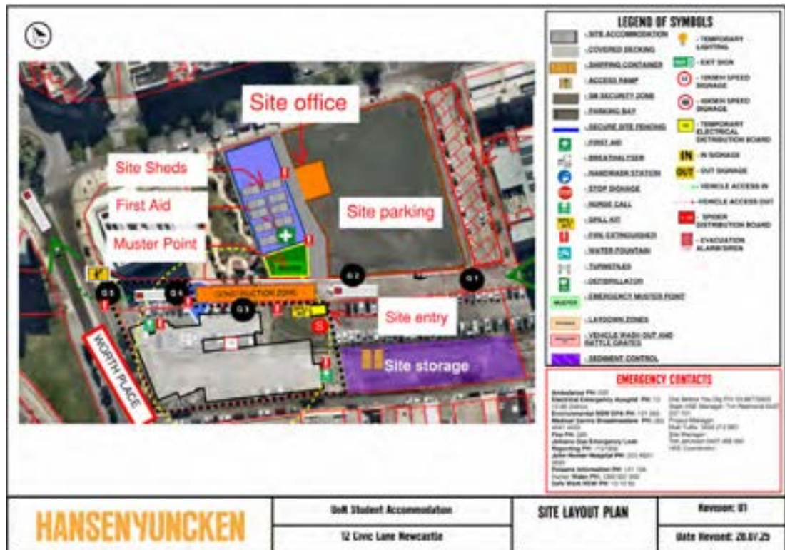
Figure 1: Site Layout Plan
