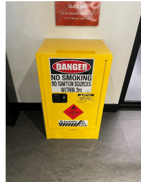
Hazchem cabinet in 3D printer workspace.
