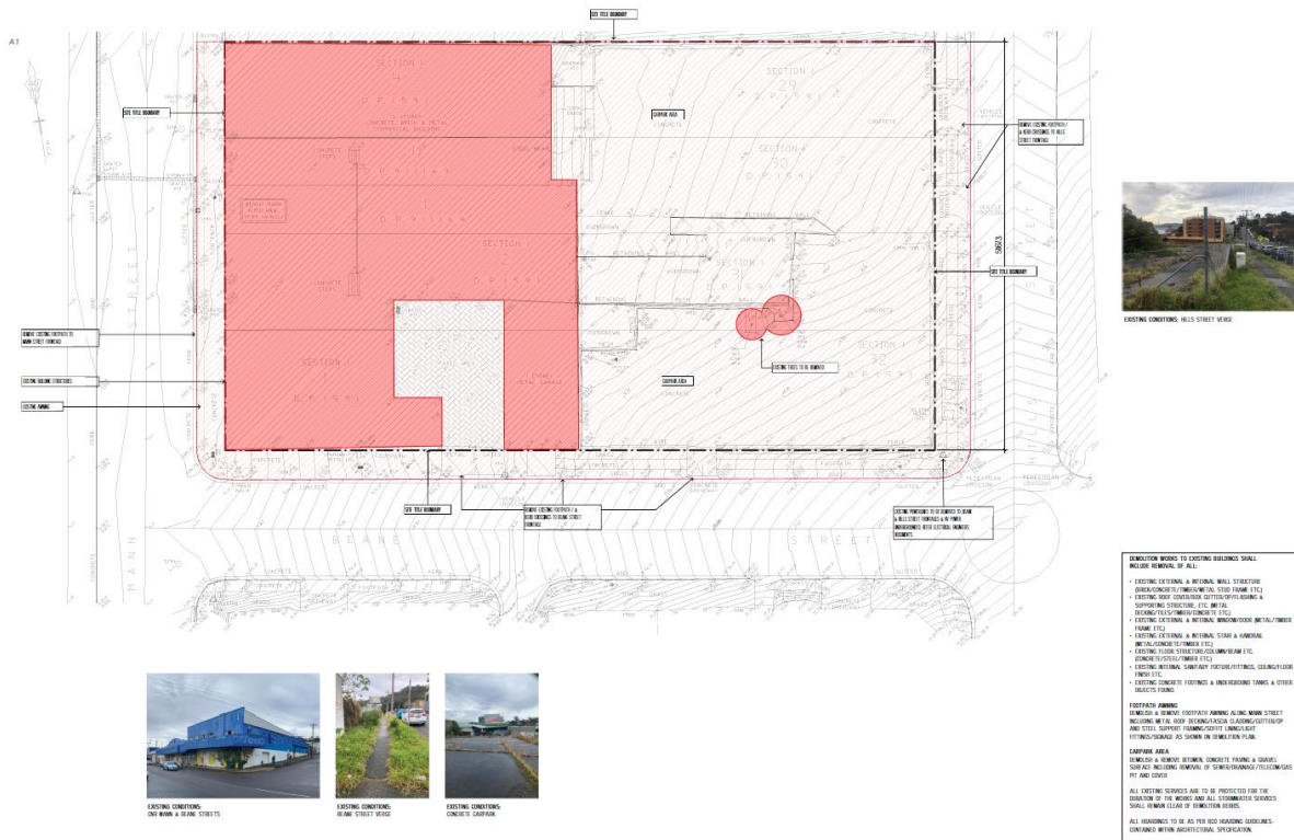
Figure 4 – Existing condition and demolition plan
