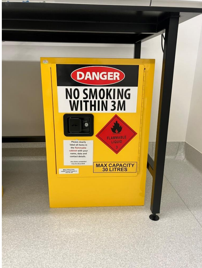
Figure 34 Chemical Storage – Flammable Liquid
