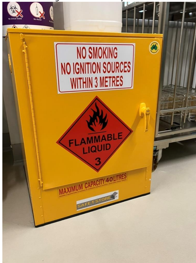
Figure 32 Chemical Storage – Flammable Liquid
