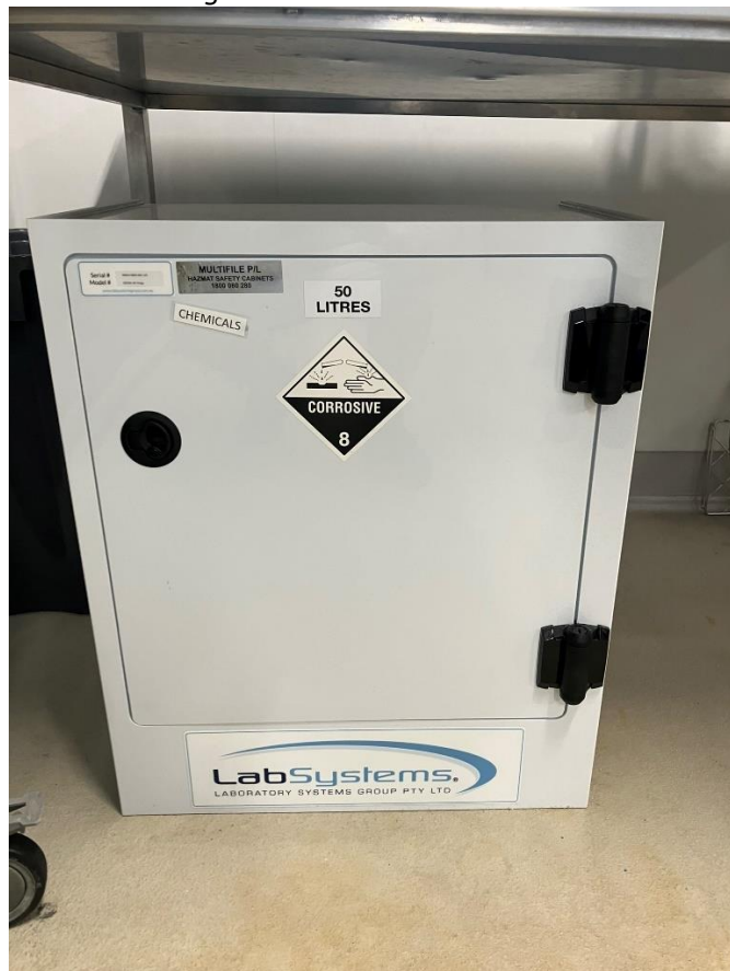
Figure 31 Chemical Storage – Corrosive
