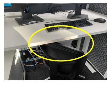
There has been a report of a sit/stand, height adjustable desk being lowered using the preset settings, the anticollision mechanism failed to stop the desk when it hit the back of a chair which had been left under the desk. This caused the computer equipment and other items on the top of the desk to be knocked over or off the desk, resulting in a near miss incident, where thankfully no one was injured.
