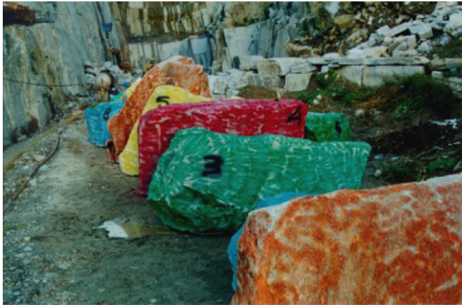
Fig. 3. View of painted blocks prior testing in order to allow proper identification of fragments.
