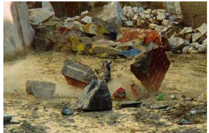
Fig. 3. View of painted blocks prior testing in order to allow proper identification of fragments.
