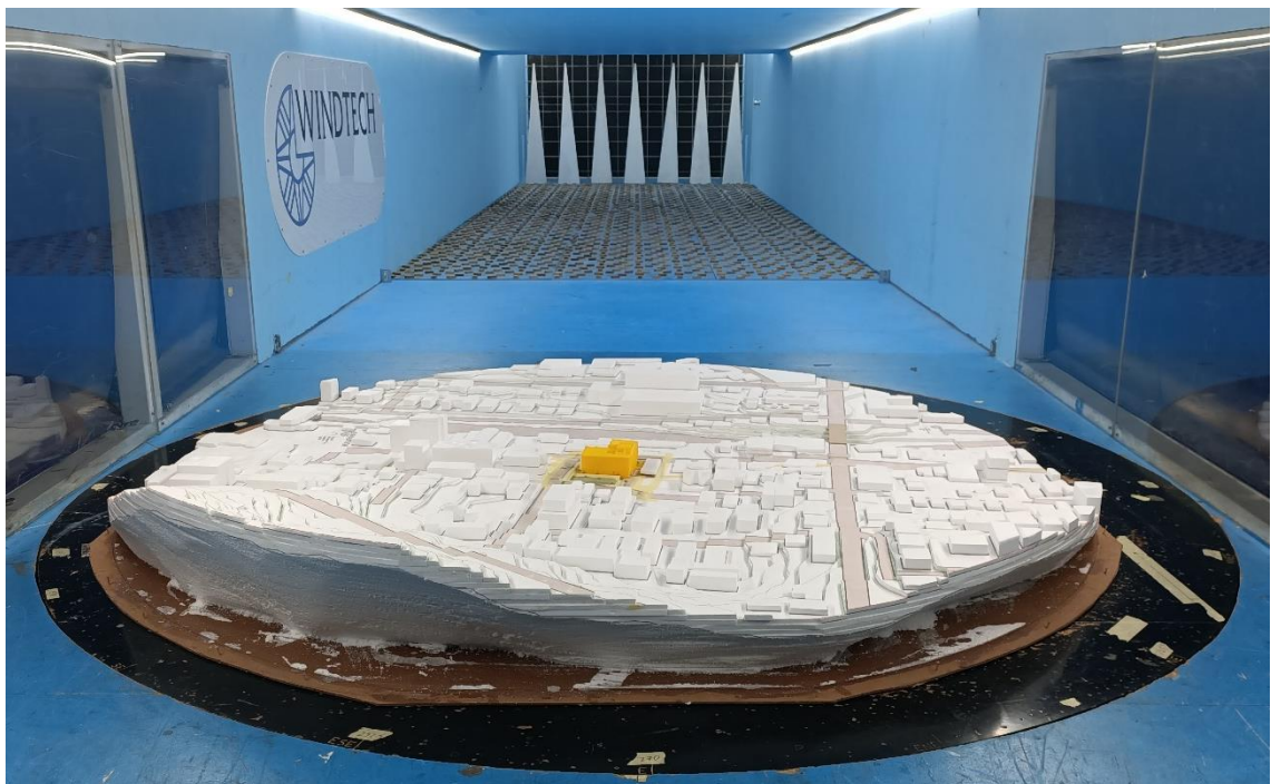
Figure 1c: Photograph of the Wind Tunnel Model (view from the east, proposed site conditions)
