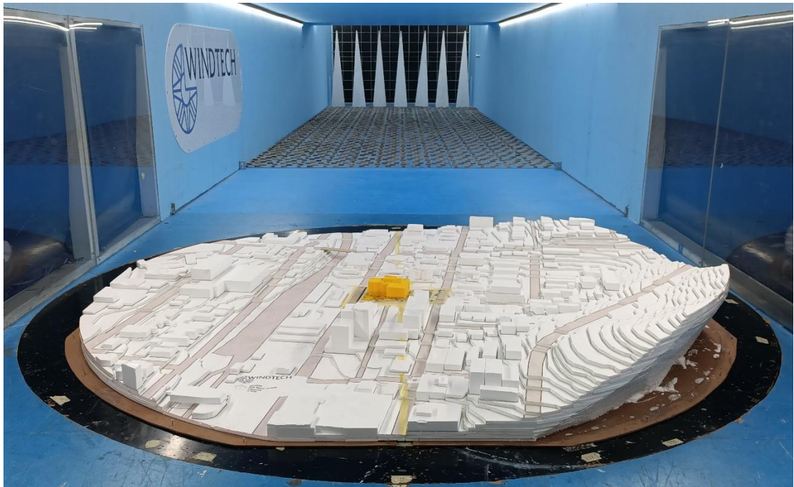
Figure 1b: Photograph of the Wind Tunnel Model (view from the south, proposed site conditions)
