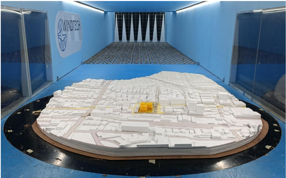
Figure 1e: Photograph of the Wind Tunnel Model (view from the west, proposed site conditions)
